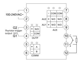
**Note:** 4~20mA linear current signal can change to 20~100mV voltage signal by connecting a 5 ohm resistor, and then be inputted from terminals 11 and 10.
