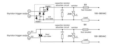
**Note 1:** According to the voltage and current of load, choose a suitable varistor to protect the thyristor. A resistor-capacitor circuit (RC circuit) is needed for inductance load or phase-shift trigger output.
